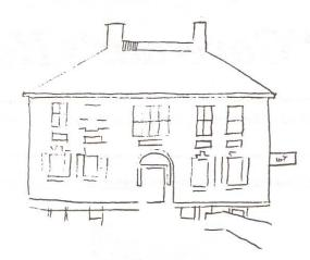
Above is a tracing of an 1826 sketch of the Governor's Mansion included in the background of a more careful drawing of the Capitol building. It shows the house as built with a fanlight over the front door and no porch. The panels are indicated, and the upper balustrade, added in 1823, also appears here.
